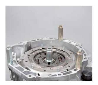
Mount the puller (KL-0500-60) with the thumb screws (KL-0500-6020) on the threaded bolts such that they are stress-free
