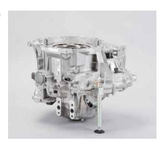
• Disassemble the retaining ring of the upper clutch disc hub (K1) using a screwdriver
