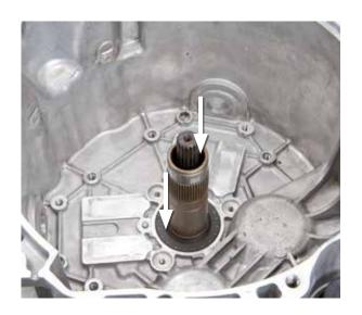
• Check that the adapter sleeves and dowel pins are securely in place
