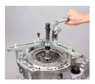
Turn the spindle via the press-in sleeve to press the clutch onto the hollow shaft; the pressing process is complete as soon as the retaining-ring groove is fully visible in one of the windows of the press-in sleeve and the amount of force required to turn the spindle increases significantly
