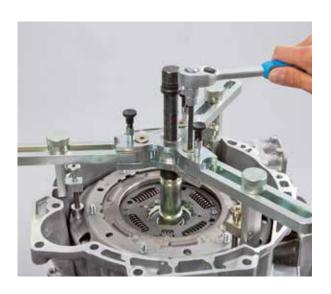
• Disconnect the clutch package by turning the spindle onto the hollow shaft
