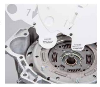
• Insert the template such that the bores on the clutch (arrow) are visible through the three large openings
