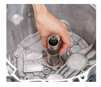
• Tighten the new screws to 8 Nm
