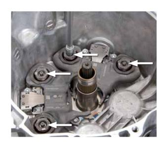
• Unscrew the mounting screws of the lever actuators
