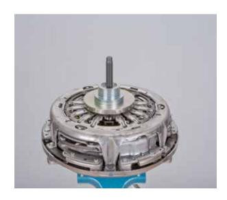
• Initially, only turn the pressure nut onto the spindle until it is touching the adapter
