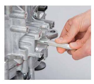
Apply an extremely thin layer of grease to the spindle of the lever actuators as well as to the shafts of the servo motors
