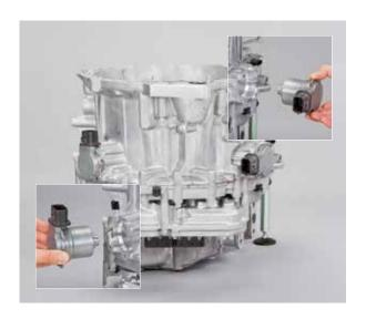
Insert the unlocking key (KL-0500-8011) with the marking (on the ribbed surface) facing upwards into the lever actuator for K2
