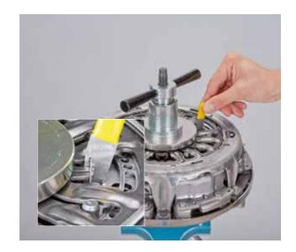
• Release and unscrew the pressure nut
