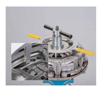
• Turn the return ring clockwise (in the direction of the arrow) as far as the stop
