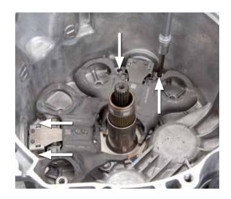
• Remove both lever actuators
