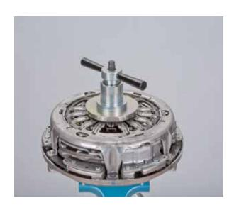
• Insert the small return ring for K1 (KL-0500-715) into the three slots of the self-adjustment ring for K1
