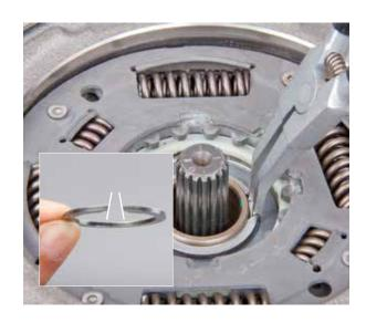
• Install the hub of the upper clutch disc (K1); the correct position is marked with a line
