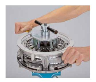
Use one hand to hold the return ring in this position, while turning the pressure nut downwards with the other hand until the pressure nut reaches the stop
