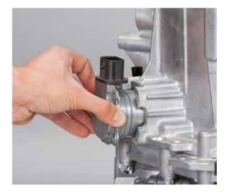
• Tighten new screws on the base plate of the lever actuators to 19 Nm
