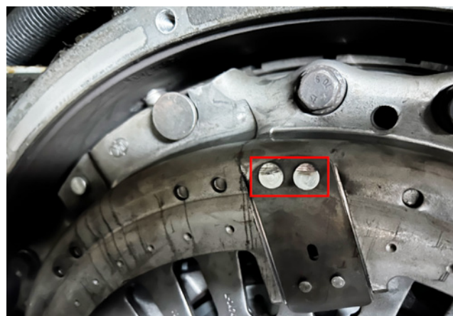
Figure 1: Material loss on the rivets due to incorrect release lever
