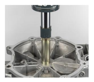
• Remove the motor-side bearing outer race in the gearbox housing using a suitable internal extractor
