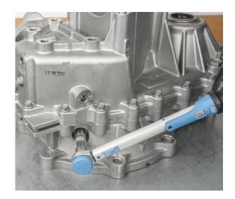
Assemble the parking lock actuator and tighten the bolts to 24 Nm
