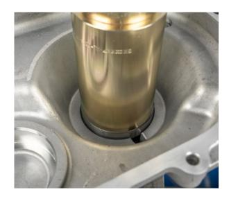
• Press off the motor-side bearing for the input shaft
