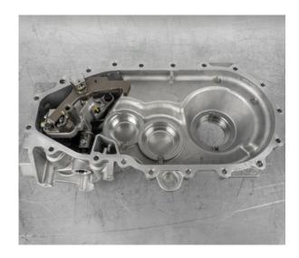
• Unscrew the bolt for the parking lock shaft
