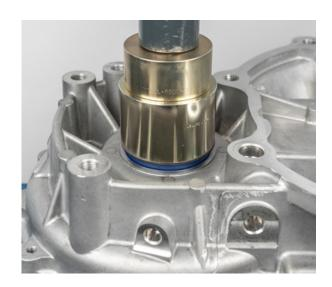
• Insert the input shaft and output shaft into the housing
