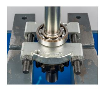
• Press on the new gearbox-side bearing for the input shaft
