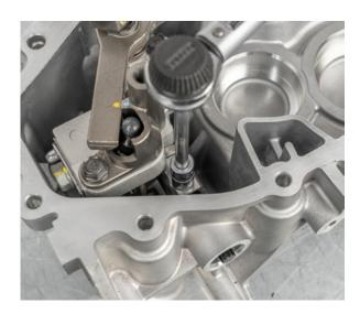
• Press a gearbox-side new outer bearing race without an adjusting shim into the gearbox housing
