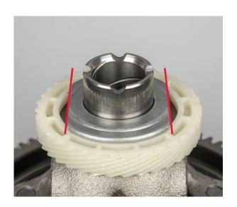
• Press the new gearbox-side tapered roller bearing onto the differential gear
