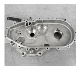
• Press the new motor-side bearing outer race into the gearbox housing
