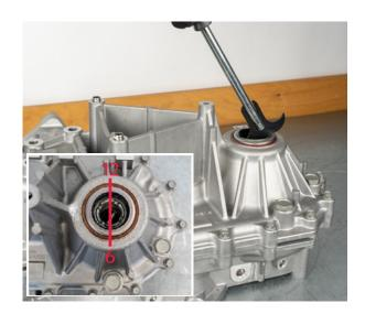
• Remove the motor-side shaft seal of the drive shaft
