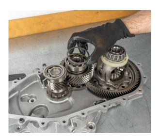
• Remove the differential gear
