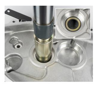
• Remove the gearbox-side bearing outer race in the gearbox housing using a suitable internal extractor
