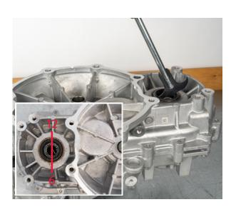
• Remove the first bolt for the parking lock
