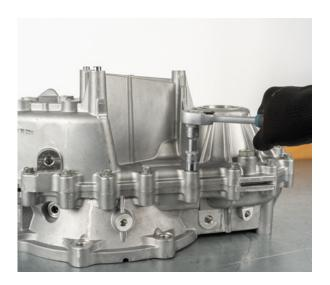
• Remove the two adjusting shims from the input and output shaft
