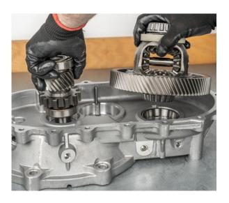
Remove the gearbox-side bearing outer race in the gearbox housing using a suitable internal extractor
