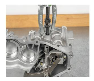
• Assemble a new shaft seal at the previous installation depth
