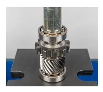
• Press off the motor-side bearing for the output shaft
