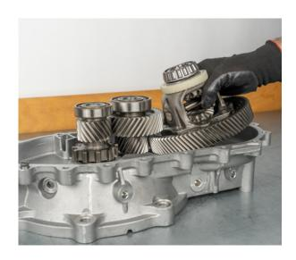
• Remove the input and output shaft
