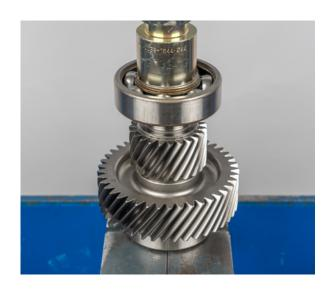
• Press off the gearbox-side bearing for the output shaft
