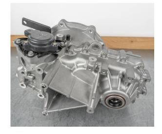
Remove the bolts and lift the parking lock actuator upwards
