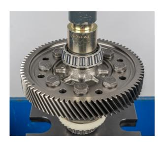
• Press off the gearbox-side tapered roller bearing from the differential gear
