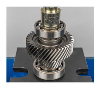
• Pull off the motor-side tapered roller bearing from the differential gear
