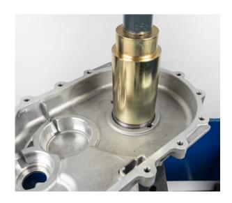
• Press in the new input shaft oil seal
