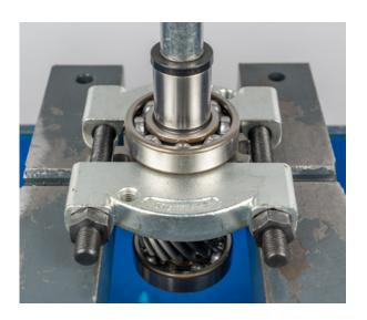
• Press off the gearbox-side bearing for the input shaft
