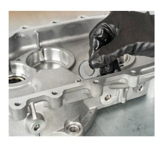
• Remove the input shaft oil seal
