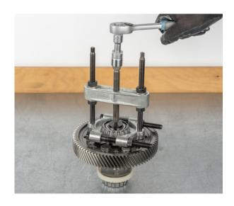
• Press the new motor-side tapered roller bearing onto the differential gear
