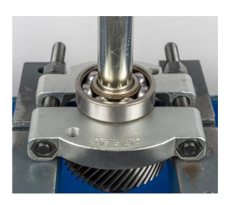
• Press on the new motor-side bearing for the output shaft
