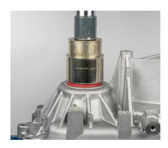
• Press in the blue, motor side drive shaft oil seal
