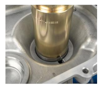
• Press in the red, gearbox side drive shaft seal
