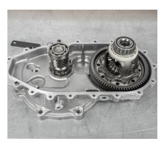
• Put on the housing cover and tighten all bolts to 15 Nm
