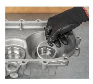
Press the gearbox-side bearing outer race back into the gearbox housing
