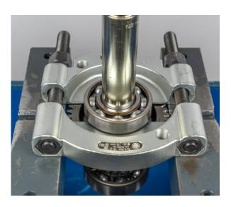
• Press on the new gearbox-side bearing for the output shaft
