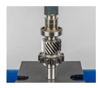
• Press on the new motor-side bearing for the input shaft
