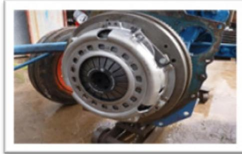
If the flywheel face has a glazed or polished appearance this indicates that repeated heating and cooling during the life of the previous clutch has created a hard skin. It is recommended that this be removed by grinding.
