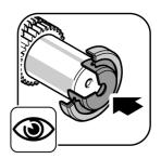
In order to guarantee that the high-performance PTFE oil seal will optimally perform its function, a minimum of 4 hours, and in some cases depending on engine application a minimum of 8 hours after assembly should pass before the shaft is moved or rotated.
