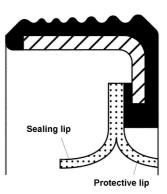
The material polytetrafluorethylene (PTFE), however, provides a solution. PTFE oil seals do withstand these extreme stresses since they
