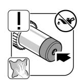
For assembly, the plastic cover is positioned such that the oil seal can smoothly slide onto the shaft. An appropriate insertion tool must be used when sliding or pressing the oil seal onto the shaft, and it must be ensured that this occurs evenly and without impact load. Otherwise there is a risk of damaging the sealing lip, and flawless sealing function is no longer guaranteed.
