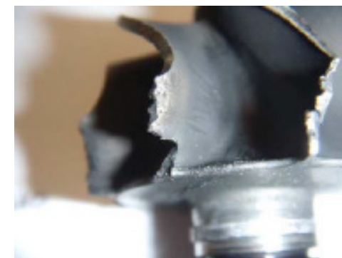
Damaged exhaust turbine
