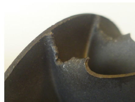
Damaged exhaust turbine
