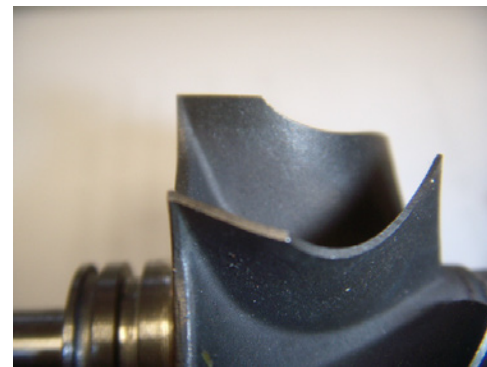
Undamaged exhaust turbine
