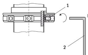
Fix the spring plate with the set screw (1) by using hex key (2) delivered by BILSTEIN.
