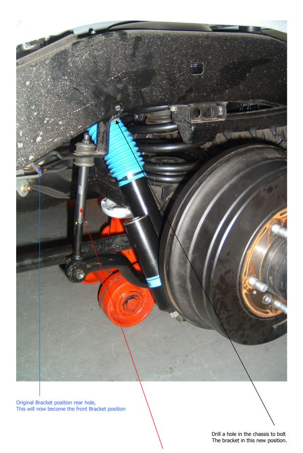
Attach extension piece MC-0077A which will be supplied and sent by KBSS LTD.
