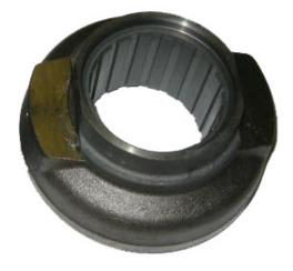
Fig. 4: Releaser with plastic slide sleeve
