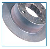
APPEARANCE Disc heavily worn with surface grooves
