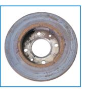
**APPEARANCE** Uneven wear of braking surfaces. Blue spots in the center of braking surface. Possible appearance of cracks
