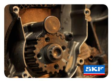
4. Lock camshaft sprocket and crankshaft sprocket using the correct tools.
