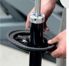
8. Ideally replace all rubber components and install these on the new shock absorber from Herth+Buss. Important: when mounting the spring cap on the suspension strut, ensure that the guide mount sits on top of the one on the shock absorber.
