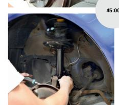
11. Finally, tighten the nuts on the top strut mounting and shock absorber fully once more. Important: it is imperative to perform an axle alignment after replacing a shock absorber, a coil spring or a top strut mounting like the ones that are also available in the Jakoparts range!
