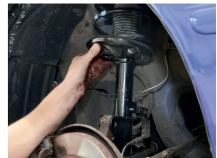
10. The assembled suspension strut with the replaced shock absorber can now be
