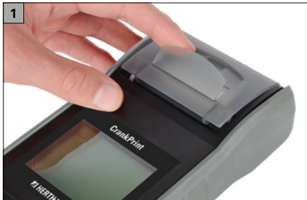
Fig. 1 Opening the cover of the paper compartment
