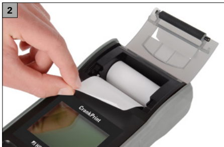
Fig. 2 Inserting the roll of paper
