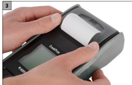
Fig. 3 Closing the cover of the paper compartment
