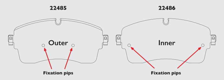
Due to these different locations of the pips, the parts are not interchangeable in the caliper. WVA 22485 is for the outer side, 22486 is for the inner side. Swapping the sides of these parts would cause the piston or respectively the fingers of the caliper to push against the pips. This could result in noise issues or an uneven wear of the friction material.
