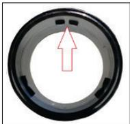
The adapter ring features three locking tabs on its inner side, one of which is equipped with a positioning groove. The connector has a corresponding locking guide. Position the adapter ring on the connector so that the positioning groove aligns with the locking guide on the connector. Then, rotate the ring 90° clockwise.
