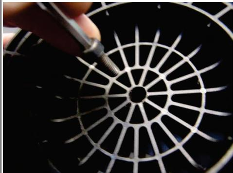
*Screw the standard end stops to the new end stop adapters using the supplied hexagon socket screw (M6x16mm) at one point (central hole).*
