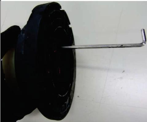
*Screw the standard end stops to the new end stop adapters using the supplied hexagon socket screws (M6x16mm) at 3 points.*
