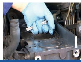
Check head height is the same and is inside tolerances, as well as side supports.
