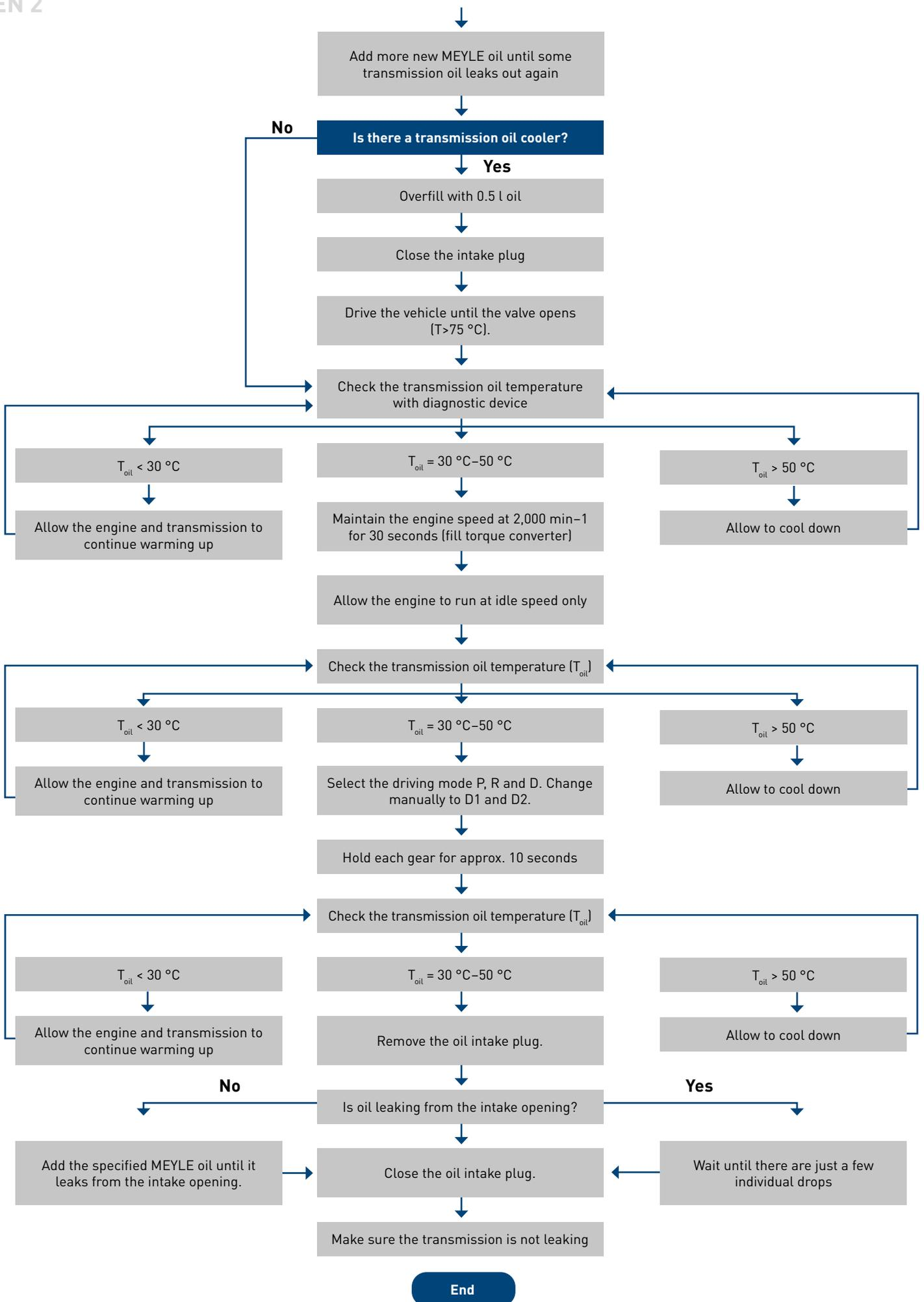
**NB:** Depending on the type of transmission, it may have a bypass valve which opens or closes the oil circuit to the oil cooler, which is why the drive should be sufficient to ensure the transmission oil temperature reaches at least 75 °C. After the drive, allow the transmission to cool down, check the oil level again and correct if necessary.
