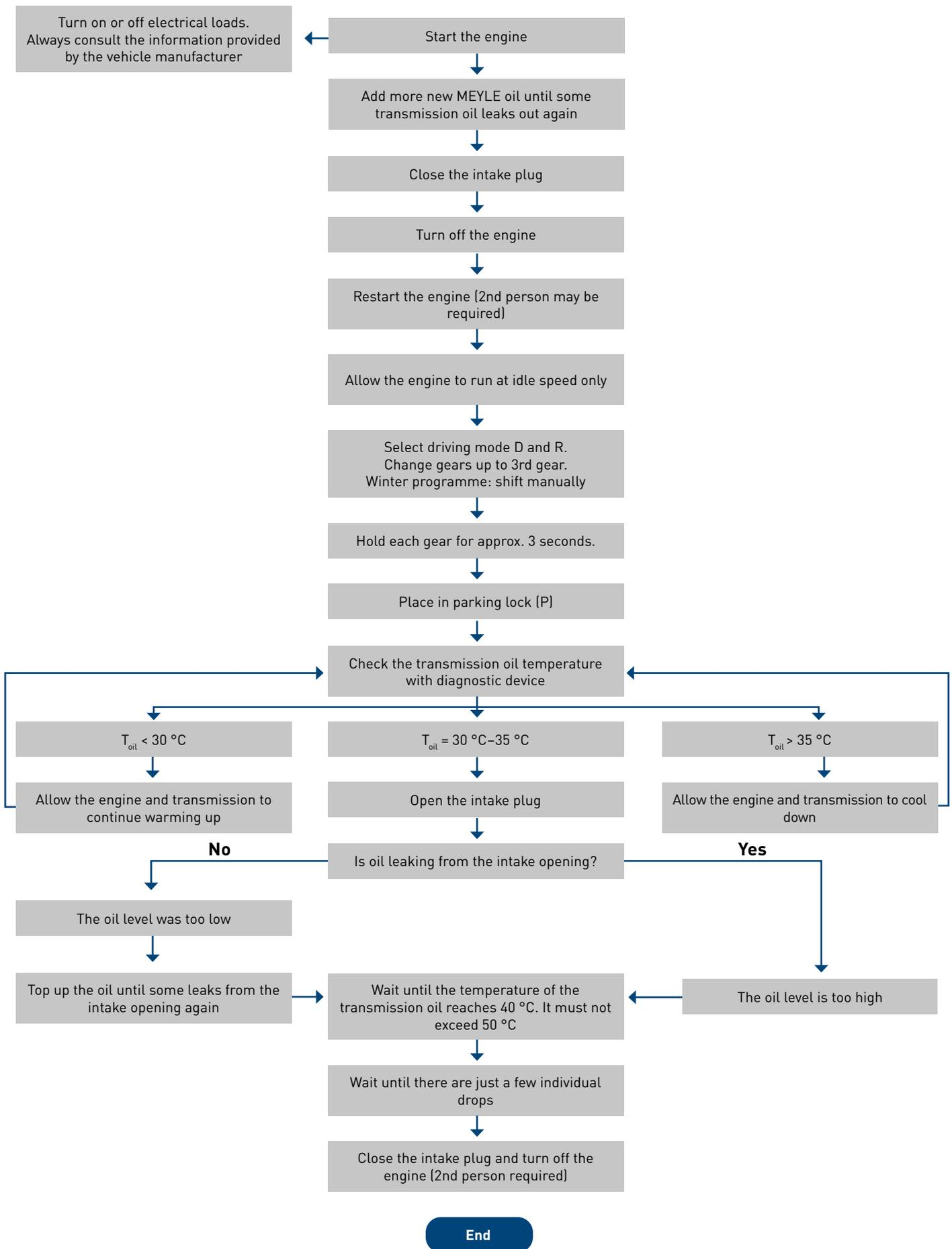
**NB: Depending on the type of transmission, it may have a bypass valve which opens or closes the oil circuit to the oil cooler, which is why the drive should be sufficient to ensure the transmission oil temperature reaches at least 75 °C. After the drive, allow the transmission to cool down, check the oil level again and correct if necessary.**
