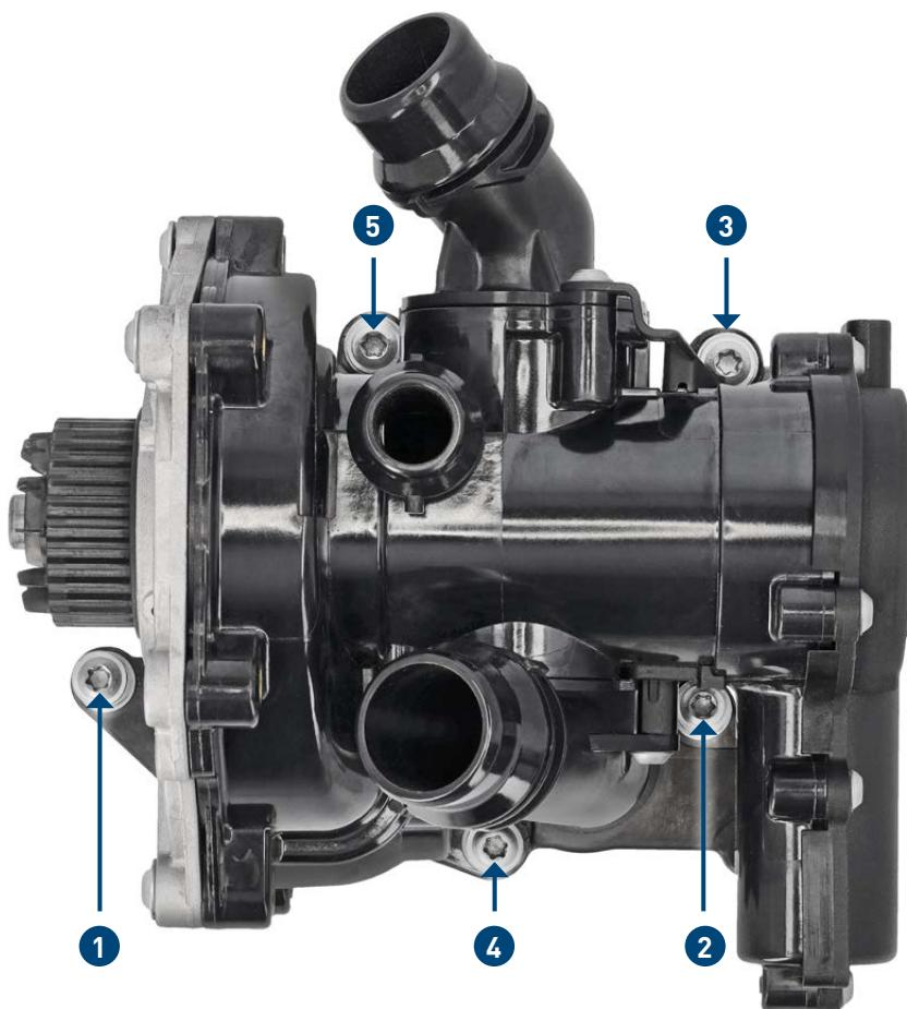
**EN:** Observe the sequence and tighten to 9 Nm
