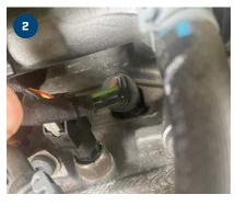
You can identify the pressure sensor glow plug by the fact that a 4-pin connector is attached to it.
