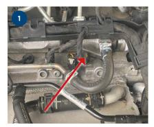
When it comes to 4-cylinder VAG engines, the pressure sensor glow plug is installed at the third cylinder.
