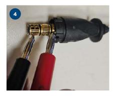
Attach a voltmeter to the top and bottom contact of the connector.
