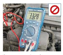
If you measure a voltage of approximately 3.3 V, the glow plug is not compatible with this vehicle.
