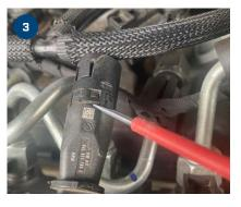
Remove the protective cap at the front with a small screwdriver.
