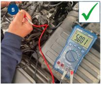
The displayed voltage must be in the range between 4.8 and 5.2 V.
