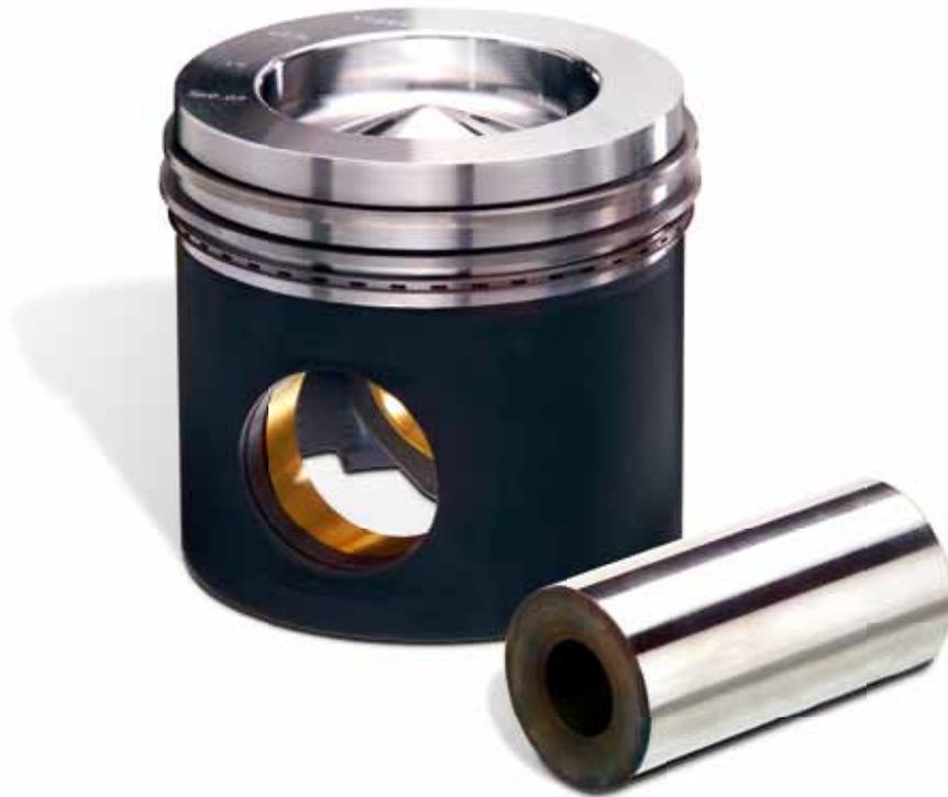
The steel piston crown guarantees minimum wear. The reduced clearance of the top land combined with the steel-guided rings enables a constantly low oil consumption. Longer service life and favourable exhaust emissions are the result.
