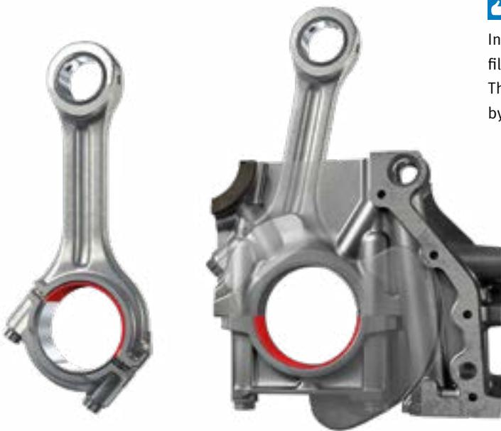
Pressure-loaded side of connecting rod and main bearings
