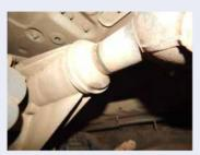
Original dust cover with smaller drain-hole
