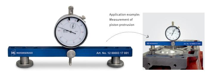
When reconditioning and assembling engines, some important amounts of protrusion on components must be adjusted, if necessary. Especially when assembling pistons, cylinder liners and valves, the protrusion/clearance must be adjusted or reworked if necessary.
