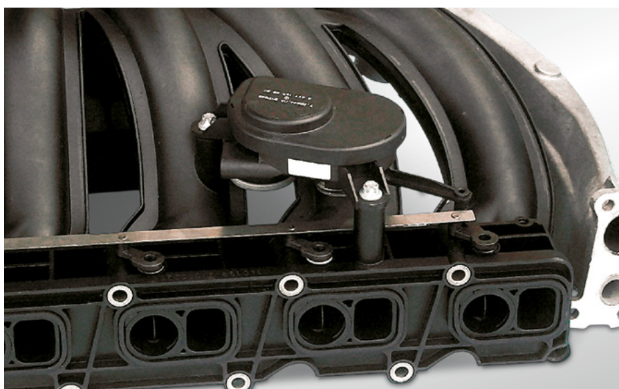
Fig. 41: intake manifold with tumble flaps and EAM-i
