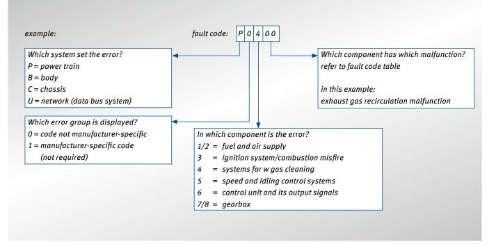
*Fig. 10: structure of the fault codes*
