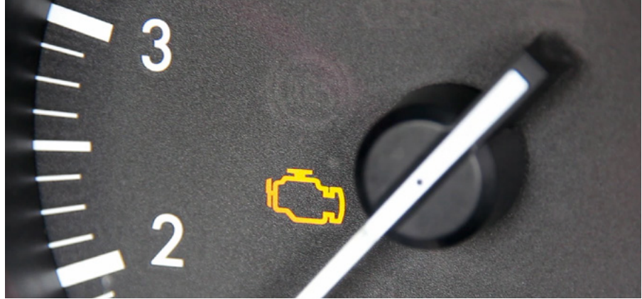
Fig. 6: malfunction indicator lamp (MIL)
