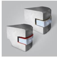
Dirt that reaches the combustion chamber settles in the ring grooves where it causes abrasive wear in the ring grooves and at the piston ring flanks. This results in excessive ring height clearance and consequently to a deterioration of the guidance of the piston rings in the ring grooves. The rings will become bent during use and start to flutter. If the rings are severely worn at the sides, they can break.
