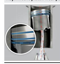
Bent connecting rods, which often occur as a result of engine damage, cause the piston to run at an angle in the cylinder. The piston rings consequently take on an elliptical form and no longer rotate in the piston. This results in uneven wear and ring flutter.
