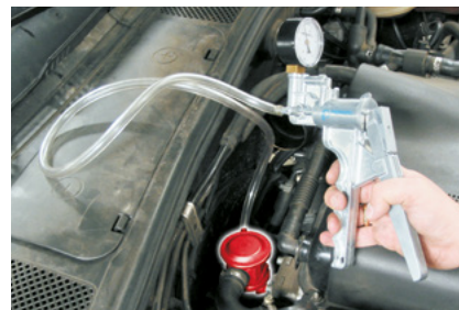
Pneumatic components are easily checked using simple tools.
