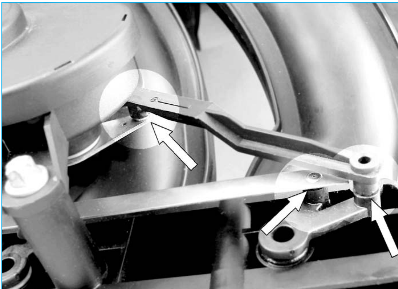
Joints between EDM-i and tumble valves
