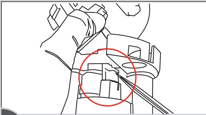
**7** DESCONECTAR EL CONECTOR INTERIOR PRESIONANDO LA PESTAÑA CON AYUDA DE UN DESTORNILLADOR.
