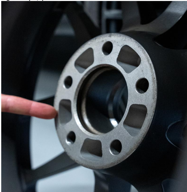
Fig. 2: Gaps / pockets in the wheels used:
