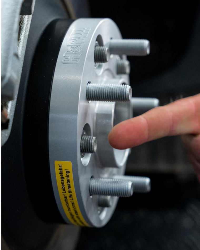
Fig. 1: Protrusion of the original stud bolts after installation of the wheel spacers:
