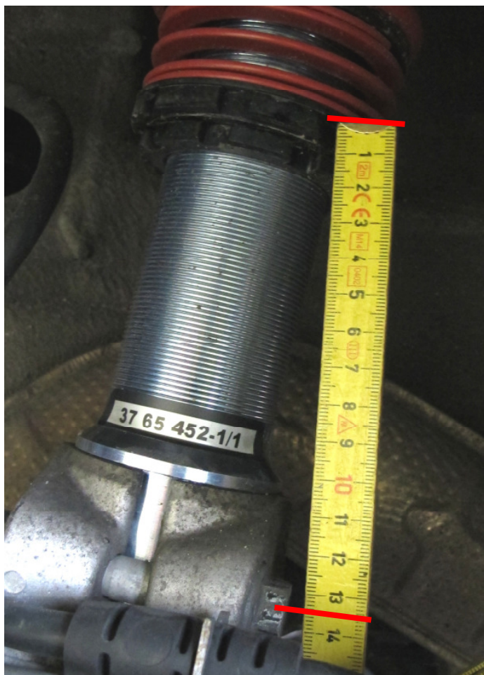
Pic. 2: adjustment dimension rear axle
