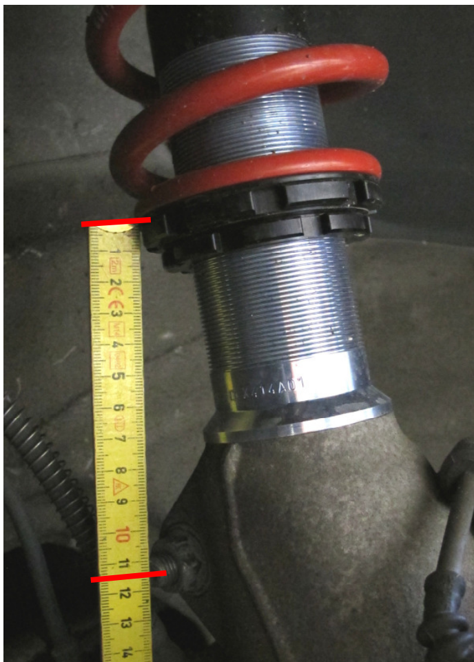
Pic. 1: adjustment dimension front axle
