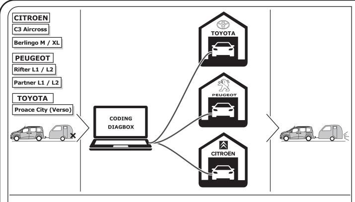
The activation of the trailer functions has to be carried out using the CITROËN DIAGBOX as follows:
