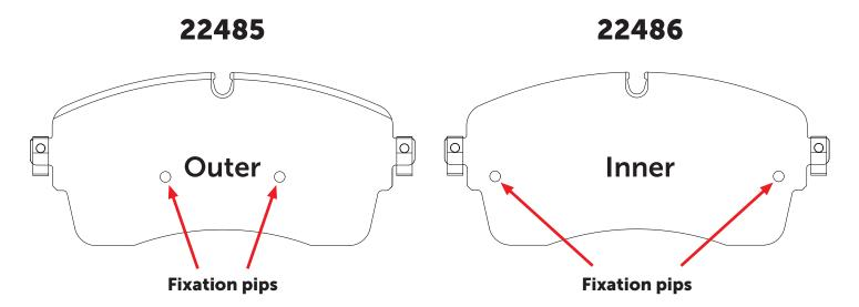
Due to these different locations of the pips, the parts are not interchangeable in the caliper. WVA 22485 is for the outer side, 22486 is for the inner side. Swapping the sides of these parts would cause the piston or respectively the fingers of the caliper to push against the pips. This could result in noise issues or an uneven wear of the friction material.
