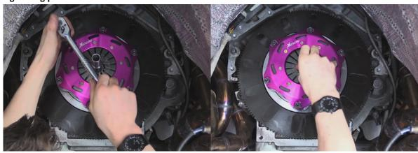
11. Finally, torque the bolts to 31Ft.lbs/41Nm.
