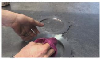
2. Apply a small amount of spline grease (supplied) to lubricate the spline in the hub of the friction discs. Insert the alignment tool or the input shaft of the gearbox into these hubs several times in different orientations to ensure that the grease is spread evenly. Ensure that the input shaft has a fine film of grease where the discs run along the spline, however make sure to remove any large drops of grease to avoid contamination of the clutch.
