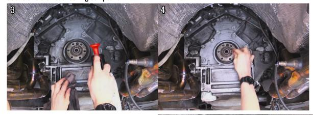
Install the new flywheel to the crank ensuring it sits true and square against the mounting surface of the crank.
