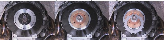
Select the next friction disc and take note of the orientation of the hub before installing it on the alignment tool. Be sure to check that the hubs do not interfere with one another in the installation order.
