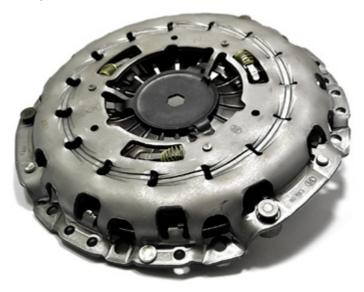
This style of retaining plate requires a special alignment tool to be inserted into the flywheel and disc before installing the cover, as pictured below.
