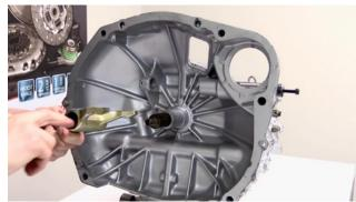
2) Re-install the clutch fork in its normal orientation and slide the cross shaft in.
