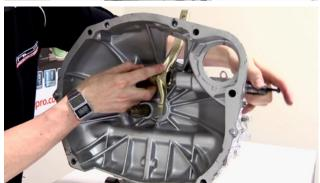
3) Install the pivot conversion block. Ensure the 2 ridges on the longer edges are sitting against the clutch fork and the threaded hole is offset towards the top. Use a small amount of thread locking compound on the bolt.
