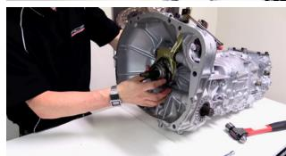
9) When the transmission is installed in the car, it's important to check that there is still a small amount of free play at the top of the clutch fork to allow the clutch to wear. This can be adjusted by adjusting either the bolt or the push rod on the conversion rod.
