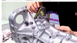
4) Install the slave cylinder using the spacers provided so that it's pushing towards the rear of the vehicle.
