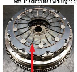
This is the hold down ring. It has 2 'handles' for removal. The other ring is a pivot ring and must remain on the clutch.
