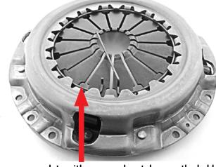
On a pressure plate with a pressed metal cover, the hold down ring will be the only visible/ removable ring.
