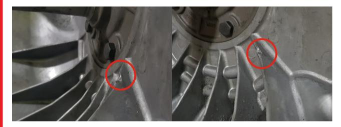
To allow for maximum fork movement and clutch wear, ACS recommends making a modification to the bellhousing ribs by grinding away a small section to avoid contact with the fork as shown in the below photos. Remove any sharp edges and burrs and test fit the fork prior to reinstallation of the clutch.
