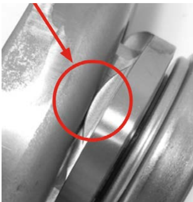
Flat fork on round bearing contact
