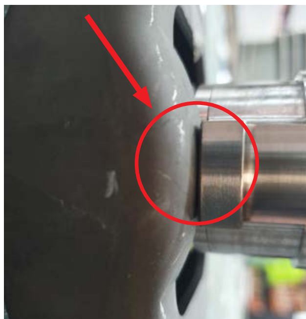
Round fork on flat bearing contact
