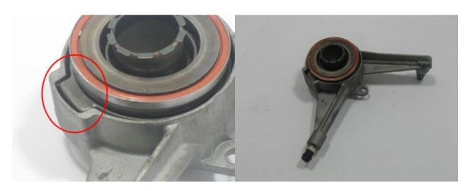
The release bearing has a guided ridge which seats in the CSC carrier. If the release bearing is fitted incorrectly the raised ridge will foul on the clutch cover causing the bearing to fail.
