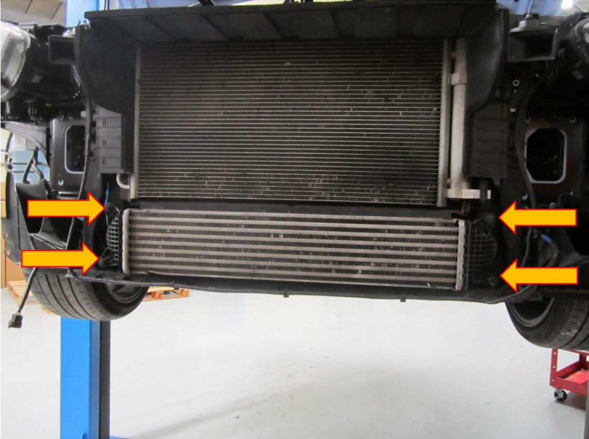
13. Using an 8mm socket and ratchet loosen the 8mm hose clamp in the same way as before, then using a 10mm socket and ratchet remove the fastener holding the OE hard pipe to the vehicle. Now remove the hose and pipe as one, from the vehicle.
