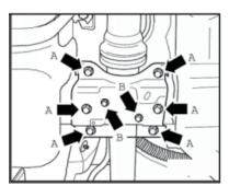
Keep the center bearing bracket in center of the lateral stoppers (arrows)
