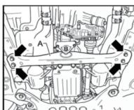
Move the gear truss sideways until the threaded holes of the center bearing and the slotted holes of the bearing bracket are aligned.
