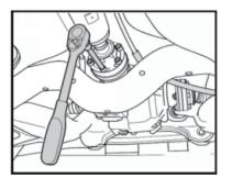
Unscrew the remaining three bolts of the propshaft on the rear axle drive
