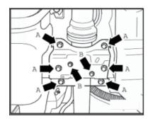
Unscrew bracket for center bearing from body –arrows A
