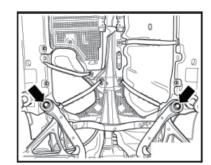
Lowering of the rear axle truss by the engine and transmission jack by the dimensions a) = 50mm.
