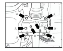
Push the rear propshaft (1) from rear axle drive (2) and swivel over flange
