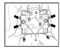
Please fix the center bearing brackt by tightening the bolts
