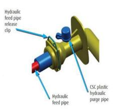
Flush the hydraulic system to ensure all contaminants and old sediment is removed from the system. Failure to flush the system may contaminate the new CSC and cause premature failure of the CSC, which is not covered by the warranty.
