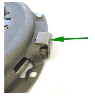
Remove 3off clips after bolting the Cover Assembly to the Flywheel
